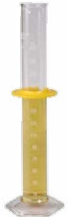
**PROBETA CON DOBLE ESCALA CLASE B ASTM**
